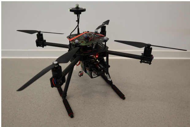
Fig. 5. Customized Holybro X500 with a Pixhawk Cube Orange flight controller, external receiver for position data, and reflective markers.
