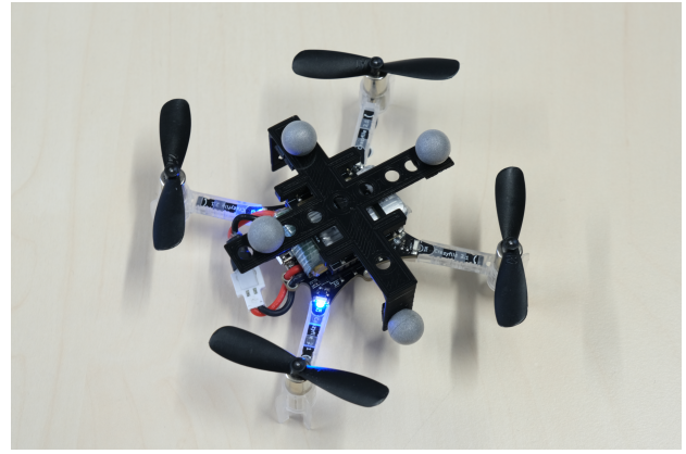
Fig. 3. Crazyflie 2.1 quadrotor with reflective markers mounted on a 3D-printed expansion deck.
