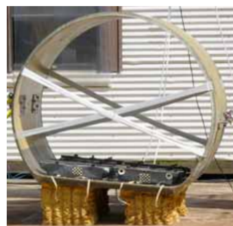
(b) Deployed Energy Absorbers in Crushed State [33]
