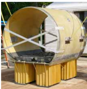
(a) Deployed Energy Absorbers in Pre-Crushed State [33]
