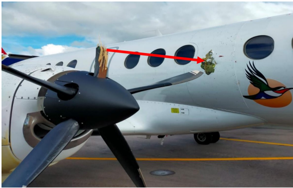
(a) Propeller detachment resulting from a birdstrike: The damage on a BAE Jetstream 41. 6
