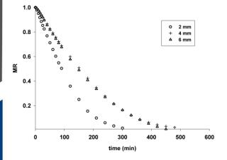
Figure 2. Moisture profile for conventional oven drying of Jerusalem artichoke slices under the effect of slice thickness change
