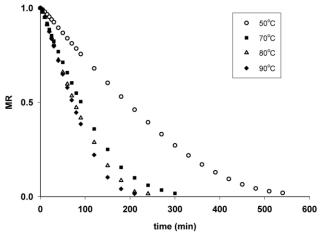
Figure 1. Moisture profile for conventional oven drying of Jerusalem artichoke slices under the effect of temperature change
