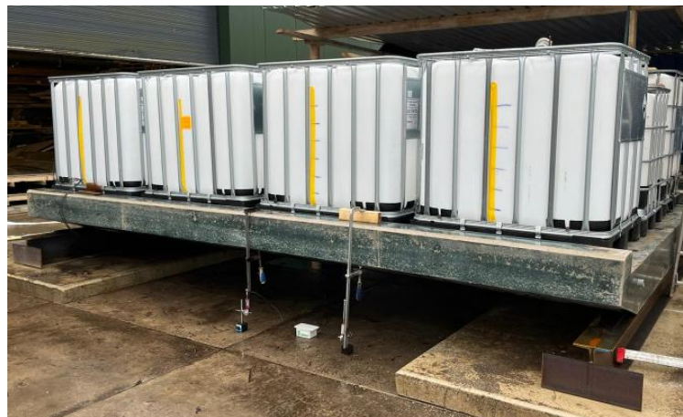
Figure 9-7 Test-setup full scale load
