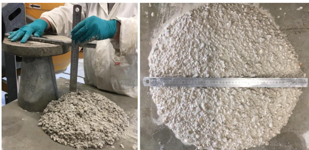
Figure 4-1 Initial slump (left) and initial flow (right) of a type of URBCON concrete
