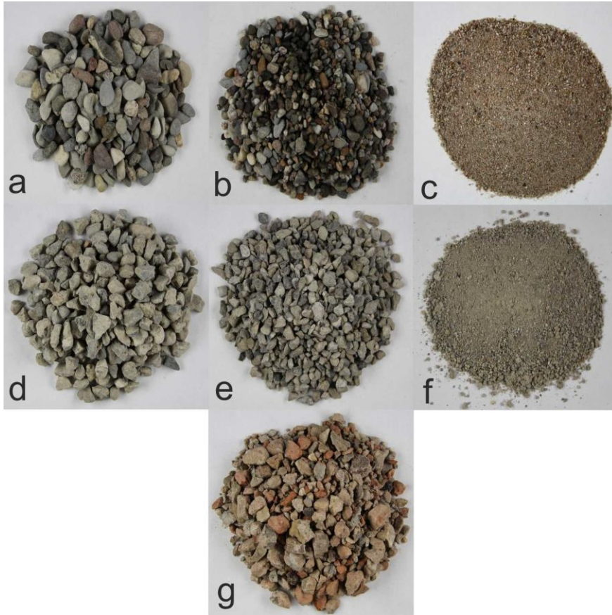
Figure 2-16 Natural (a-c) and recycled aggregates (d-g) used in the URBCON project (courtesy RPTU)
