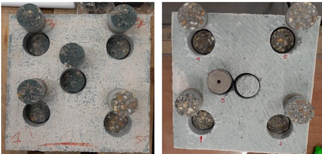
Figure 5-17 Direct tension bond testing - failure mode aspects
