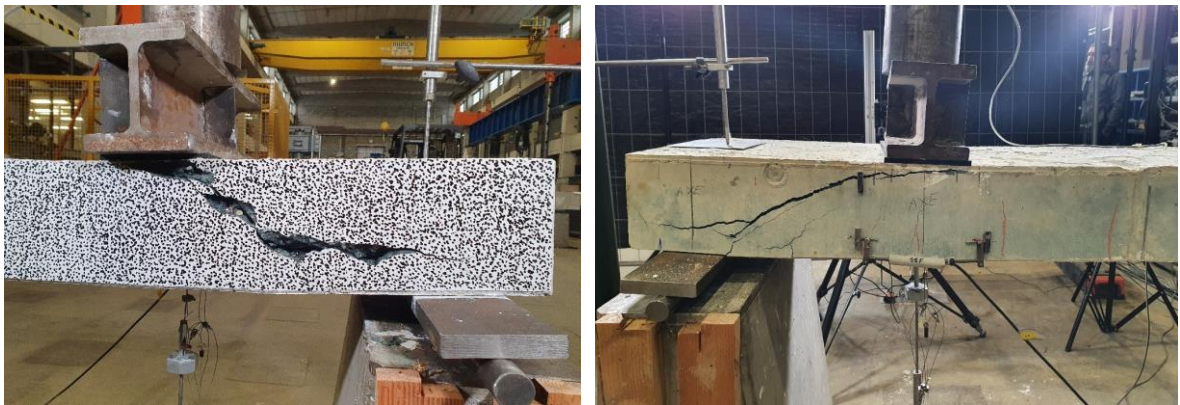
Figure 5-10 Shear tests on slabs: observed critical shear crack at failure
