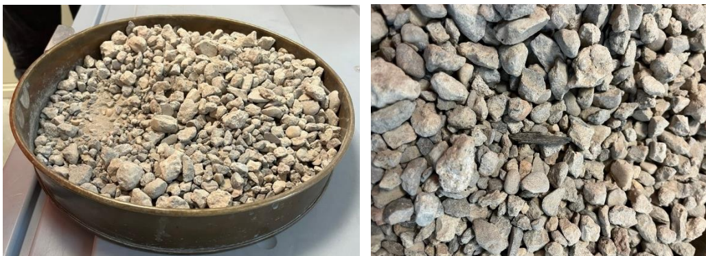
Figure 9-3 Recycled aggregates having some contamination
