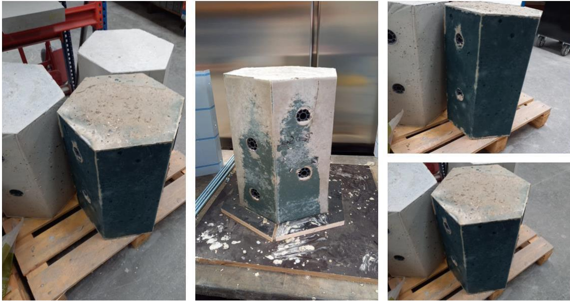
Figure 9-28 Hexagons made of different URBCON concrete types for a modular bench (note the darker colour of demoulded specimens, that disappears after a few days)
