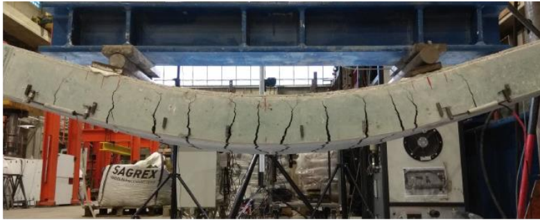
Figure 9-6 Crack pattern under bending load
