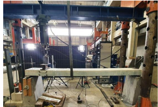
Figure 5-6 Test set-up (dimension in mm, not on scale) of flexural load tests (top) and shear load tests (bottom)
