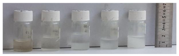
**Figure 2.** Visual determination of the precipitation intensity in five NADES samples from the left: 0%, 0-5%, 20-50%, 50-80% and 80-90%.
