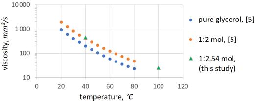
**Figure 4.** Temperature dependence of kinematic viscosities for betaine: glycerol blends. Values for pure glycerol and 1:2mol betaine:glycerol formulation were calculated from the data reported elsewhere [5].
