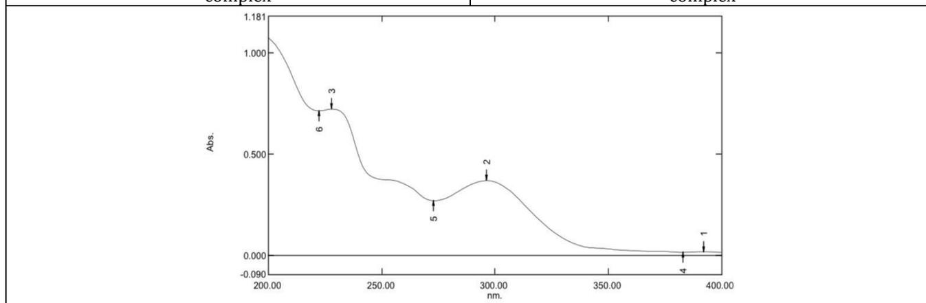
**Figure 6** Spectrum of telmisartan and HPβ-CD complex
