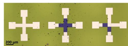
IV characterization of metal layers and Nb:STO with van der Pauw and Kelvin test structures
