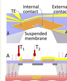
**Planar microthermoelectric generators (μTEG)** based on Si-compatible TE oxide thin films
