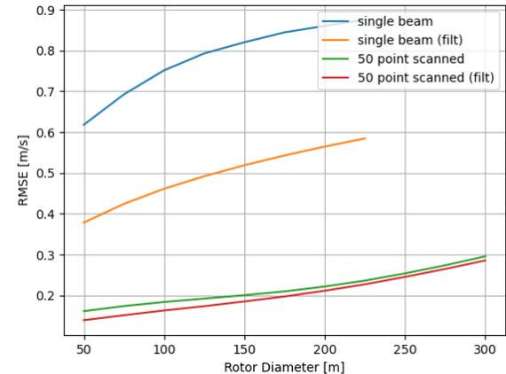
(Results using code from Simley *et al*, IEA WIND Task 32 Workshop #2, 2016, illustrate that single-beam is feasible for smaller rotors but that scanning/multibeam is required for modern turbines)
