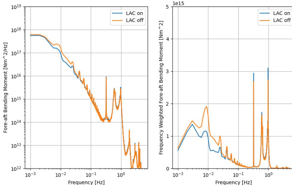
Left: power spectra of tower base fore-aft bending moment
