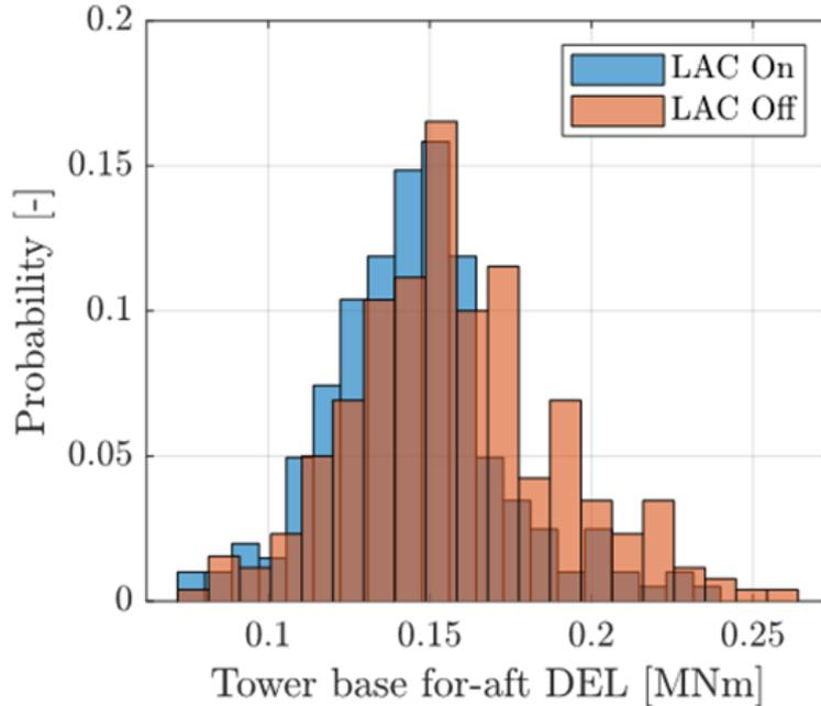
Overlapping histograms of DEL for each 1,000-second period clearly illustrate the DEL reduction when LAC is applied
