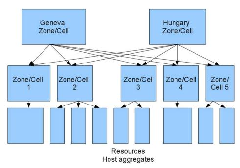
Each physically separated region has an IaaS entry point which knows about all zones and cells at all sites, and each zone has two parent instances. This way, the two entry points are equivalent, and can be hidden behind a (load balanced) DNS alias.
