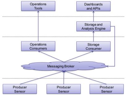
Data is produced by multiple sensors distributed across the data centre, data is transported through a messaging infrastructure allowing aggregation, data is stored and analysed in a large data store, and finally data is made available via tools, dashboards, and APIs tailored for operations and for analysis/historical queries.
