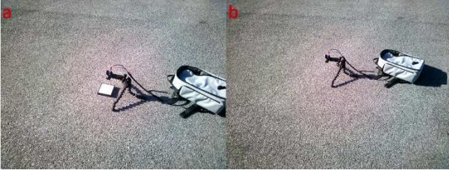
Fig. 2. Measurement setup with a tripod mounted optical fiber 0.20 m above an asphalt surface, with the RS-3500 within the bag. (a) Incoming spectral radiation is estimated from measurements of the rectangular white Lambertian panel. (b) Outgoing spectral radiation is measured directly from the surface. The spectral reflectance (2) is the fraction of the outgoing radiation to the incoming radiation.
