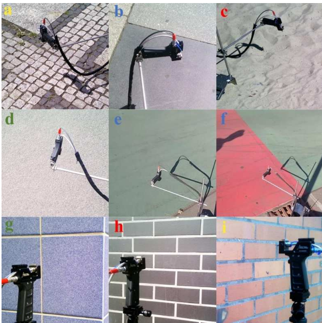
Fig. 4. Examples of materials included in the HS library, collected from the area of Berlin. (a) Stones, (b) Granite, (c) Sand, (d) Asphalt, (e-f) Painted-Asphalt, (g) Ceramic-Tiles, (h-i) Bricks. More information about the materials shown in this figure can be found in Table I. The labels show measurements from four neighborhoods in Berlin, color-coded as follows: red for Charlottenburg, yellow for Neukolln, green for Lichtenberg: green, blue for Mitte.
