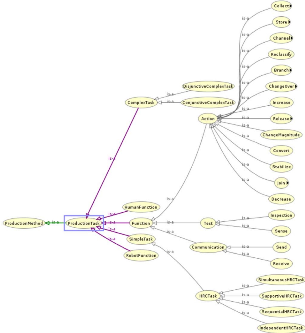
Fig. 3. Taxonomical structure of production tasks with the integrated Taxonomy of Function [12]. Please note that the concept Action is a particular type of Function and falls under the namespace of SOHO. This concept is therefore different from the concept DUL:Action defined within DUL.
