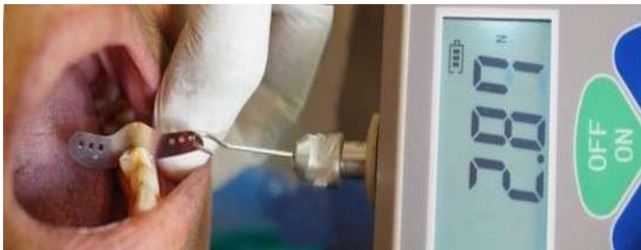
Figure 5:- Evaluation of Proximal Contact Tightness using Digital Force Gauge and 0.05mm metal strip at Cementation appointment.
