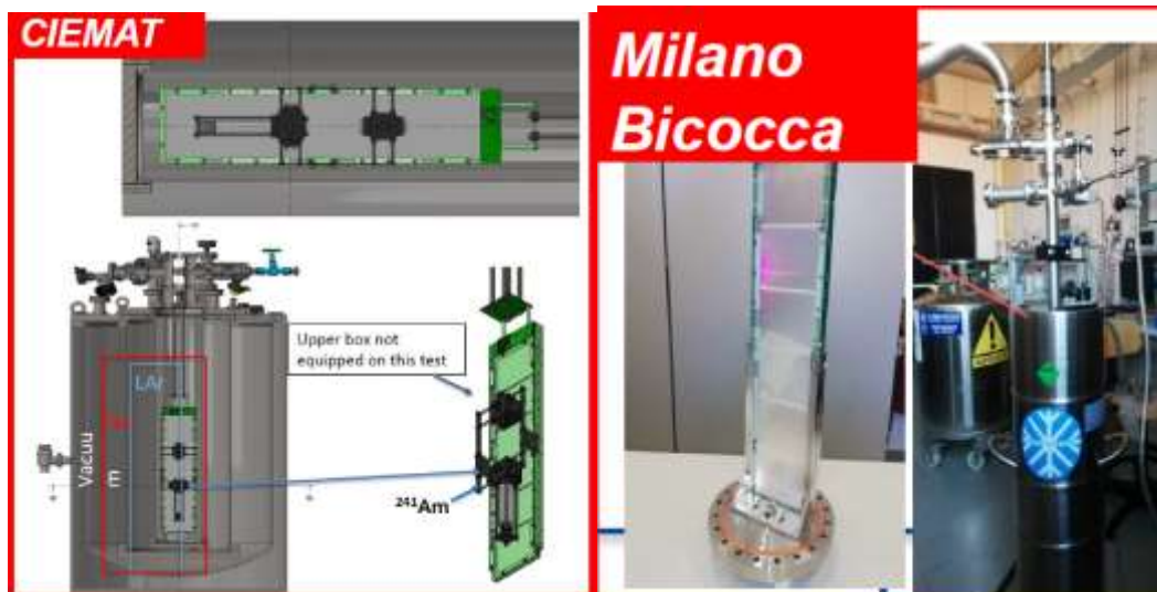
Figure 5 Test stand at CIEMAT and INFN-MIB for the X-ARAPUCA of ProtoDUNE II
