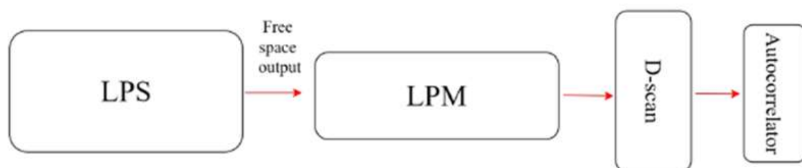
Figure 2: LPS, laser pulse source; LPM, laser pulse management module; D-scan, dispersion management module and characterization of the laser pulse by dispersion scanning.
