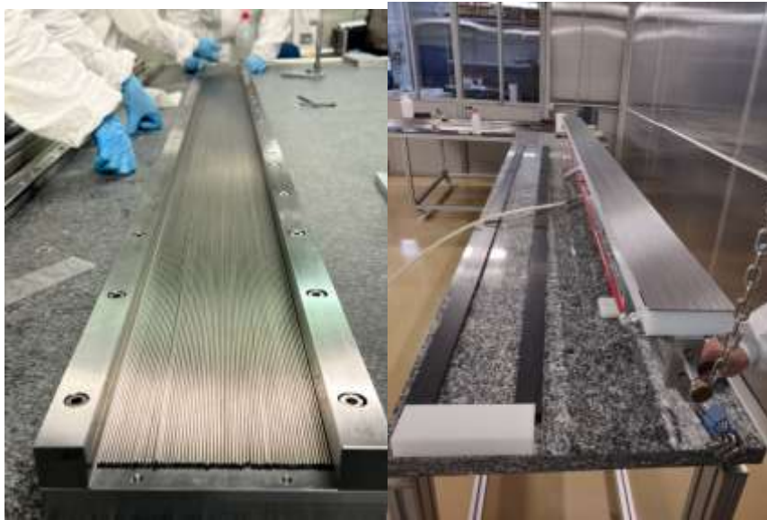
Figure 3: Left: The assembly reference structure anchored to the granite table, with a layer of tubes already in position. Right: Jig for tube handling and positioning.
