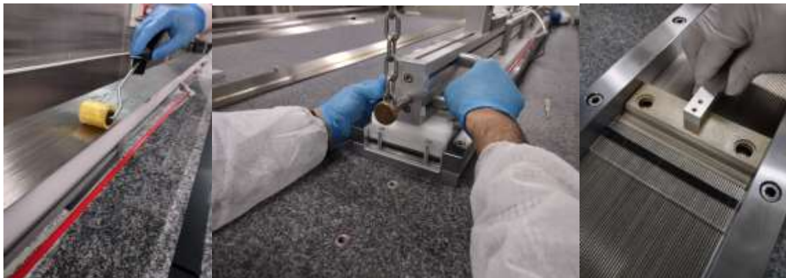
Figure 4: Left: the glue is rolled in small amount on the tube surface while the tubes are kept on the jig by means of the vacuum system. Center: the jig allows you to position the layer of tubes on the top of the previously stacked tubes. Right: The plexiglass plates equipped with a double-sided tape and kapton, used to hook the tubes with the vacuum system.
