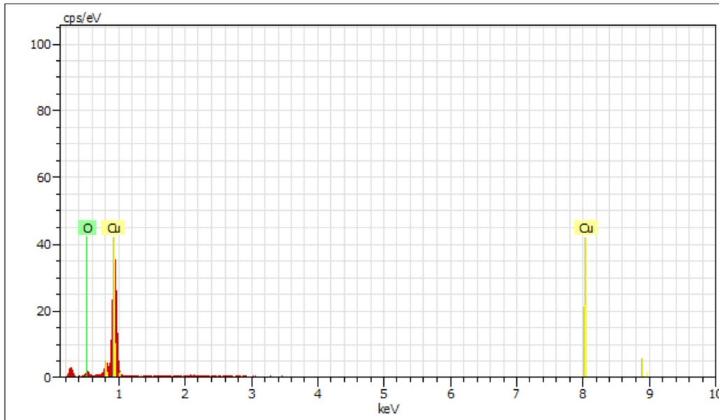
**Figure 3** Energy Dispersive X-ray Spectroscopic (EDAX) image of CuO nanoparticles
