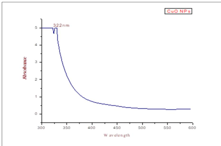
**Figure 1** UV-Visible Spectroscopic image of CuO nanoparticles
