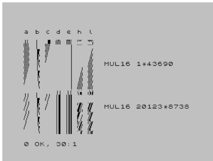
Fig. 4. The Z80 processor comes from a similar era as Fairchild’s integrated circuits, and was a foundational design to modern microprocessors. Here we display the contents of its register memory after every microcode instruction of two multiplications of 16 bit numbers, revealing the patterns created.
