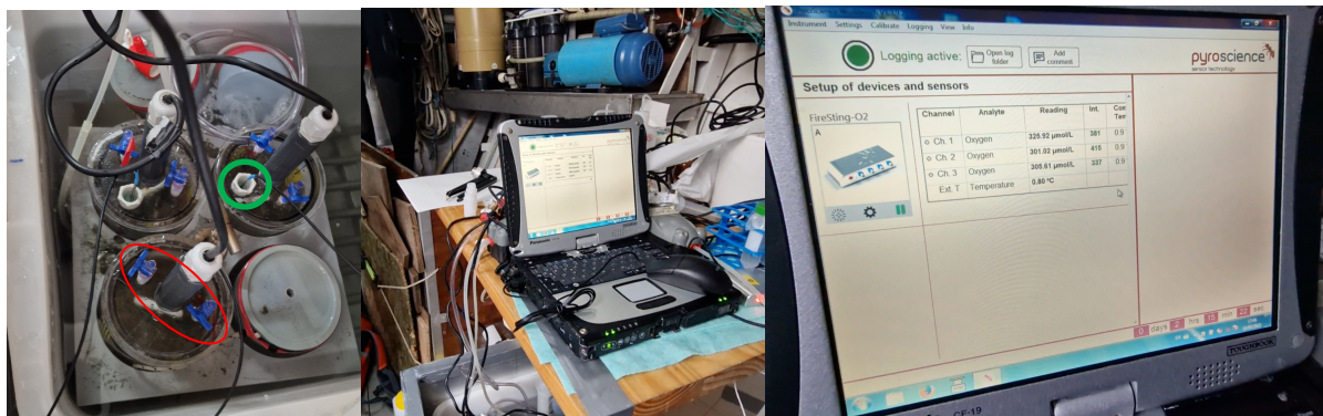
Figure 45: Incubation setup with three cores submerged in the thermostatic bath with the airtight lids operating the stirrer and hosting the optodes ports (green) and the water sampling ports (red).
