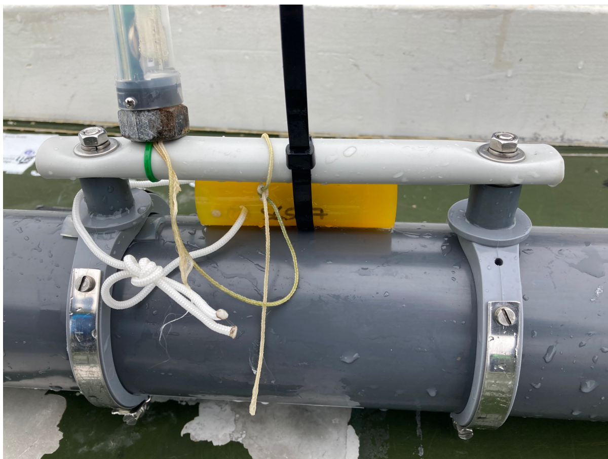
Figure 29 Details of the HOBO light and ODDI CTD sensors setup on the 2.5L Niskin. The ODDI sensor is secured in the yellow plastic tube.
