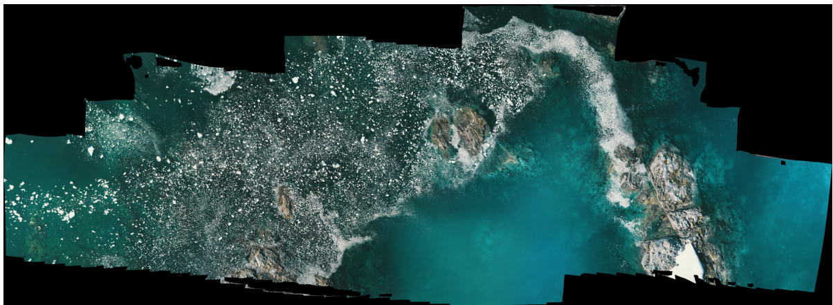
Figure 28: Orthomosaic image obtained by aligning 668 images shot by the drone (DRM_1) in Dodman Island (partial result)
