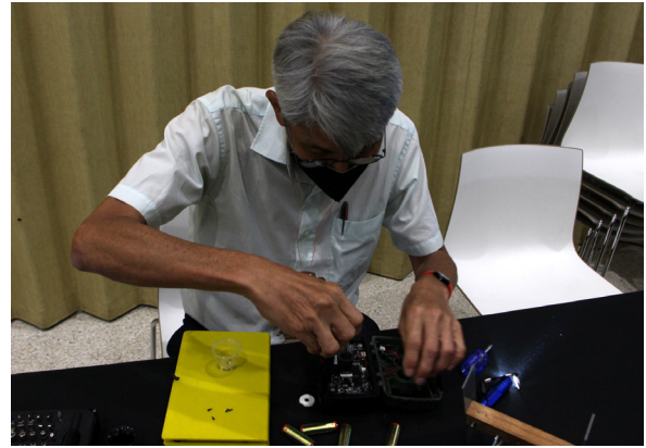
2. Harold Tay showing how to to open the case of a camera trap and tap into its triggering circuit (attribution: Laura Olalde source ; licence: CC0 )
