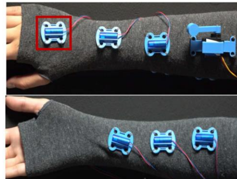
Fig. 1. The custom-made vibrotactile sleeve. Red square marks the actuator that is used to give vibrotactile feedback during the experiment.
