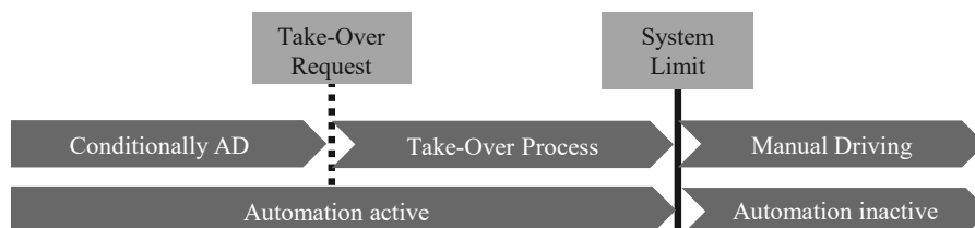
Fig. 1. Take-over process in a SAE Level 3 vehicle.
