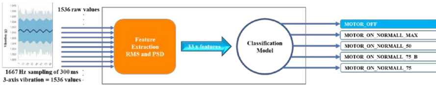
Figure 1.34 Temporal and frequency plots as input to motor classification.
