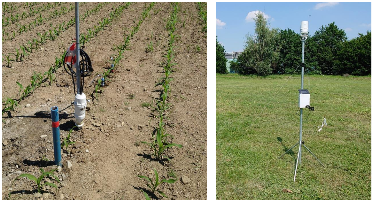
Figure 15: Sensors and devices installed: piezometer, water content probe + GSM modem, porous cups (left); agrometeorological weather station (right).
