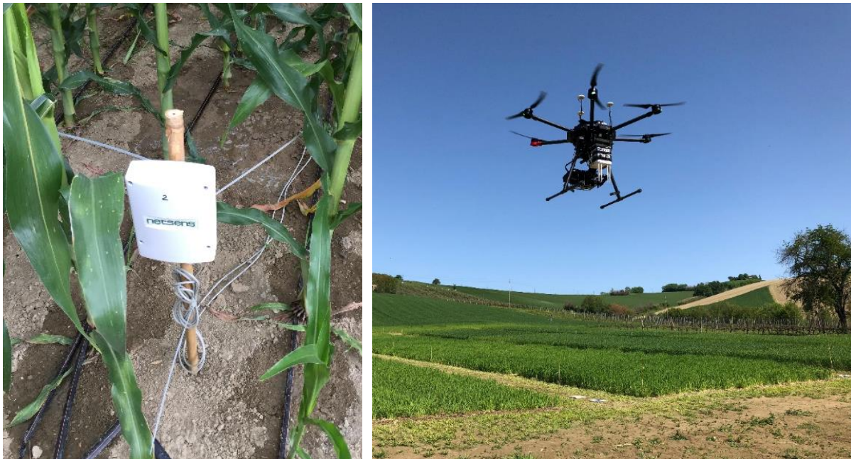
Figure 2: Ground sensors and Unmanned Aerial Vehicle to detect water stress.
