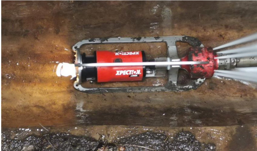
Figure 28: An iPEK XPECTION device for smart sewer cleaning.
