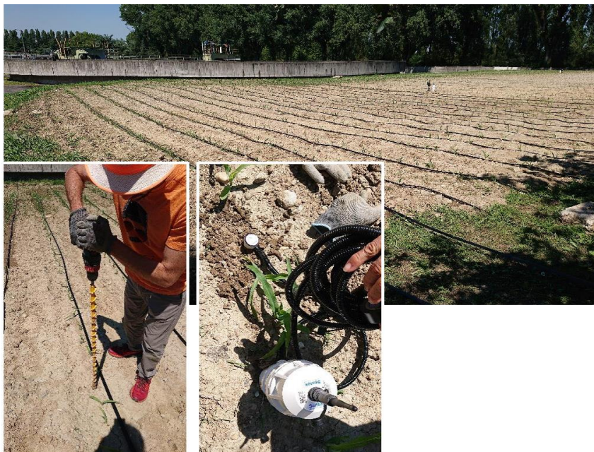
Figure 4: Installation of ground sensors within the Peschiera Borromeo test area
