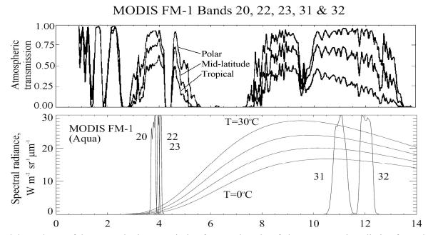
Spectral dependence of the atmospheric transmission for wavelengths of electro-magnetic radiation from about 1 to 14  $\mu$ m, for three characteristic atmospheres (above), and (below) the black-body emission for temperatures of 0, 10, 20 and 30°C, and the relative spectral response functions of the bands MODIS (Flight Model 1) on *Aqua* used to derive SST.
