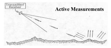
Backscatter of EMR transmitted toward sea surface from a space borne instrument.
