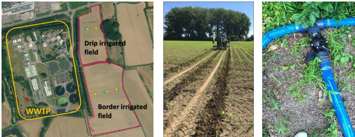
Figure 11: Overview of demo site (left), drip irrigation system installation (centre), electro-valve regulating irrigation in each sector (right)
