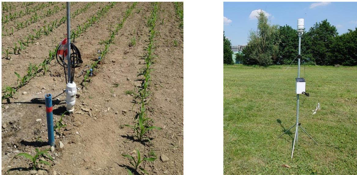
Figure 12: Sensors and devices installed: piezometer, water content probe + GSM modem (left); agro-meteorological weather station (right)
