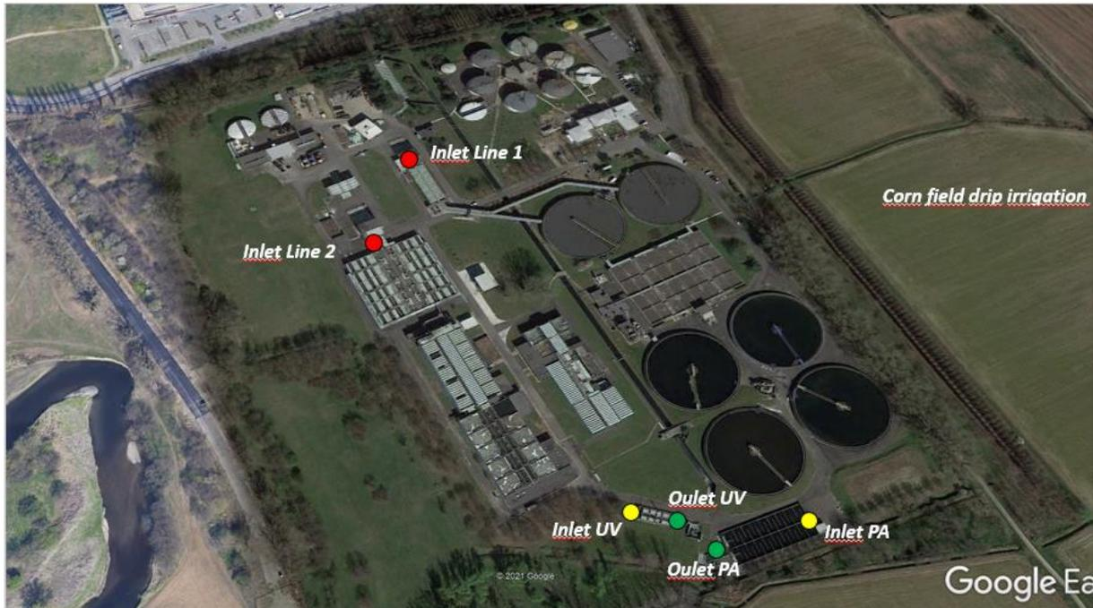
Figure 13: Sampling points of 2019-2021 campaigns from Line 1 (disinfection process by Peracetic Acid) and Line 2 (disinfection process by UV irradiation) for determination of emerging contaminants and emerging pathogens in raw and treated wastewater
