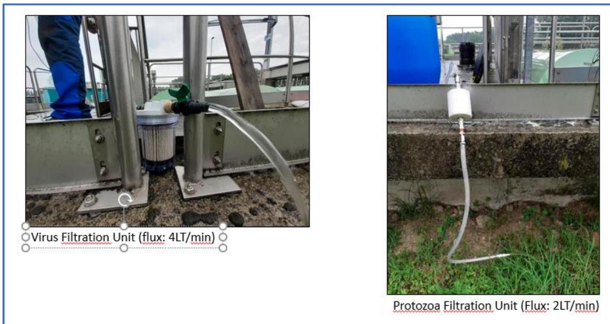
Figure 17: In situ primary filtration with collecting units for viruses (left) and protozoa (right)
