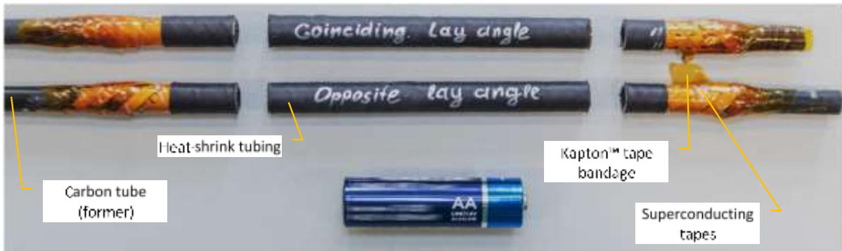
Fig. 1 Cable samples (centre) with two senses of helicity were prepared by cutting exactly 4 twist lengths from a longer hand-made cables.
