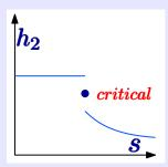
Fig. 17.14 – Downstream flow height as a function of the step height.
