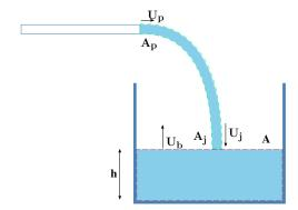
Fig. 5.7 – Filling of the bucket and choices of the deformable control volumes for example 5.3.
