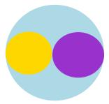
Fig. 4.66 – The cross section of the interface. The purple color represents the maximum heavy liquid raising area. The yellow color represents the maximum lighter liquid that "goes down."
