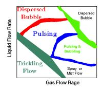
Fig. 16.7 – A dimensional vertical flow map under very low gravity against the gravity.
