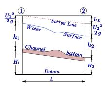
Fig. 17.25 – The energy line and liquid surface line with the energy lost. As can be observed the flow is subcritical.
