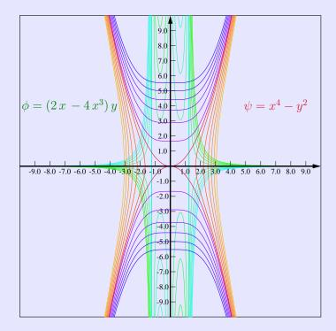
Fig. 12.5 – Stream lines and potential lines for Example 12.4.
