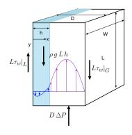
Fig. 16.17 – General forces diagram to calculated the in a two dimension geometry.
