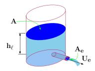
Fig. 7.2 – Discharge from a Large Container with a small diameter.
