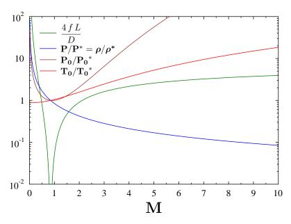
Fig. 14.18 – Description of the pressure, temperature relationships as a function of the Mach number for isothermal flow.
