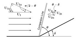
Fig. 15.3 – A typical oblique shock schematic.
