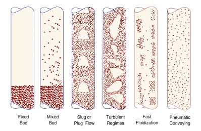
Fig. 16.10 – The flow patterns in solid-liquid flow.
