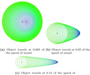
(c) Object travels at 0.15 of the speed of sound.
