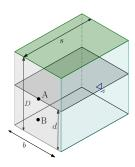
${\bf Fig.~4.49}-{\rm Rectangular~body~floating~in~a~liquid~for~stability~analysis.}$
