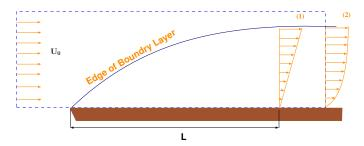
Fig. 5.9 – Boundary Layer control mass.
