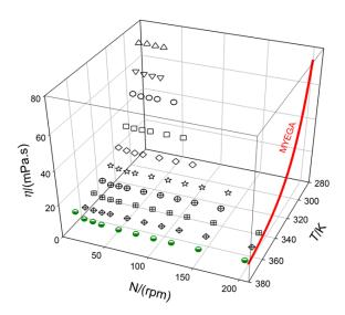
Fig. 1.10 - Cotton seed oil kinetic viscosity in 3-D as a function of pressure and temperature.The symbol  $\eta$  should be  $\nu$  as figure made by non fluid mechanics after Nieves M. C. Talavera-Prieto, Abel G. M. Ferreira, Anto nio T. G. Portugal, and Ana P. V. Egas The kinetic viscosity affected strongly by the temperature and it depend on the chem-
