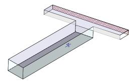
${\bf Fig.~4.55}$  – T shape floating to demonstrate the 3D effect The rolling creates yaw. To correct the energy method, it suggested that a new stability potential energy should build similar to velocity potential that is discussed in this book on potential flow. The following definition should be adapted. The stability potential is defined as
