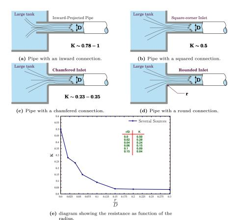
Fig. 11.8 – These figures exhibiting the entry loss into pipe from a large tank based on the initial condition (geometrical configuration). In the literature there is a dispute on the exact values. For example, Crane Co. contents that inward connection is k=0.78 while Kotowski et al found that K=1. Any value in this range seems reasonable. See at the end of the Chapter for references. Any increase of r/D beyond the value of 0.15 seem fruitless.
