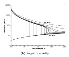
Fig. 1.6 – Nitrogen (left) and Argon (right) viscosity as a function of the temperature and pressure after Lemmon and Jacobsen.
