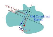
Fig. 4.48 – Arbitrary body rotates in  $\theta$  and the buoyancy centroid rotates in  $\alpha$ . The brown  $\alpha$  shows the case of stable scenario. The purple depicts the large  $\alpha$  not stable case.
