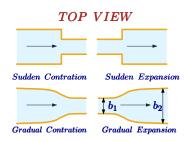
$\label{eq:Fig.17.20} \textbf{Fig. 17.20} - \text{expansion and contraction} \\ \text{top view in gradual and abrupt.}$
