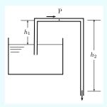
Fig. 6.15 - Flow Through a Siphon
