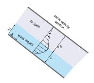
Fig. 8.23 – Flow of liquid in partially filled duct.
