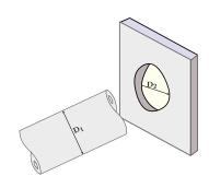
Fig. 9.1 – Fitting rod into a hole.
