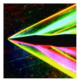
Fig. 15.9 – Color-schlieren image of a two dimensional flow over a wedge. The total deflection angel (two sides) is  $20^{\circ}$  and upper and lower Mach angel are  $\sim 28^{\circ}$  and  $\sim 30^{\circ}$ , respectively. The image show the end–effects as it has thick (not sharp transition) compare to shock over a cone. The image was taken by Dr. Gary Settles at Gas Dynamics laboratory, Penn State University.
