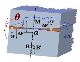
Fig. 4.56 – Stability analysis of floating body.
