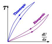
Fig. 1.8 – Thixotropic and Rheopectic fluids with the hysteresis and the time depended.
