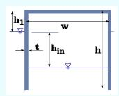
Fig. 4.37 – Schematic of a thin wall floating body.
