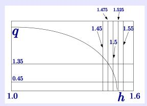
Fig. 17.23 – The Flow Rate for Contraction Exercise. Ex. 17.4. Note that  $h_1$  is not the actual height but rather height if the flow rate was same based on section 2. Notice, the solution can be obtained analytically and numerically in many methods. With knowledge of the height, the velocity can be calculated as
