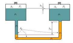
Fig. 4.7 - Schematic of sensitive measurement device.
