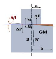
**Fig. 4.62** – Calculations of GM for abrupt shape body.
