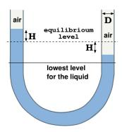
**Fig. 7.5** – Flow in an oscillating manometer.
