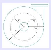
Fig. 5.17 – schematic of single stage centrifugal pump.
