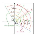
Fig. 12.8 – Two dimensional Vortex free flow. In the diagram exhibits part the circle to explain the stream lines and potential lines.
