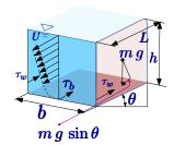
Fig. 17.7 – Force balance in the flow direction open channel. Notice that in this case  $\tau_w = \tau_b = \tau_0$ .
