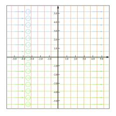
Fig. 12.6 – Uniform Flow Streamlines and Potential Lines.
