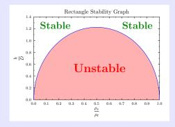
Fig. 4.50 – Extruded rectangular body stability analysis.
