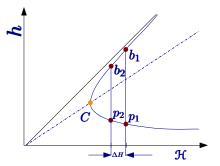
(b) Energy line with the effects of elevation change showing the two possibilities.
