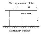
**Fig. 5.18** – Moving plate toward a fixed surface.
