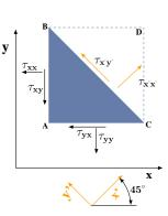
Fig. 8.10 – Shear stress at two coordinates in  $45^{\circ}$  orientations.
