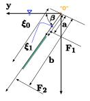
Fig. 4.22 – The general forces acting on submerged area.
