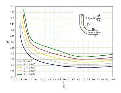
Fig. 11.11 – The resistance in  $90^{\circ}$  bend with relative roughness.
