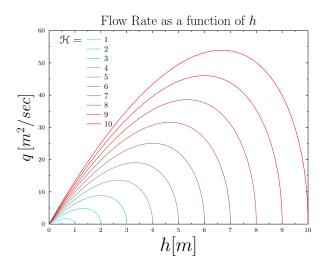
**Fig. 17.19** – Flow Rate as Function of height, h, for various,  $\mathcal H$  in the range of 1.0 to 10.0 Alternatively, all the graphs can be summarized into dimensionless equation as
