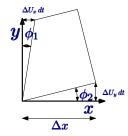
Fig. 8.13 – Schematic to explain shear angle.
