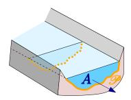
Fig. 17.8 – Constant cross section in general. Orange is the perimeter,  $\mathscr{P}$ , and the area, A, is the cross section.
