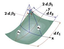
Fig. 1.17 – Surface tension control volume analysis describing principles
