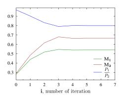
**Fig. 14.36** – Conversion of solution for given  $\frac{4 f L}{D} = 0.5$  and pressure ratio equal 0.8.
