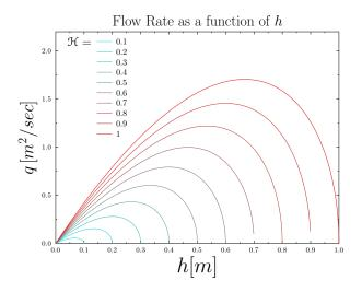
Fig. 17.18 – Flow Rate as Function of height, h, for various,  $\mathcal H$  in the range of .1 to 1
