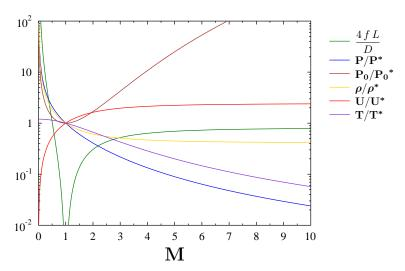
${\bf Fig.~14.20}-{\rm Various~parameters~in~Fanno~flow~shown~as~a~function~of~Mach~number.}$
