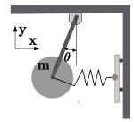
Fig. 3.20 – Pendulum attached to a fractional–less mass.
