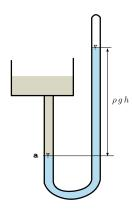
Fig. 4.3 – A schematic to explain the measure of the atmospheric pressure.
