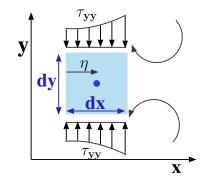
Fig. 8.7 – The shear stress creating torque.
