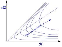
(a) Height lines for open channel as a function of the energy for various constant flow rate lines.
