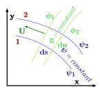
Fig. 12.3 – Constant Stream lines and Constant Potential lines.
