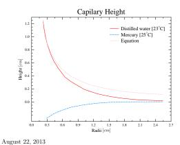
Fig. 1.26 - The raising height as a function of the radius.
