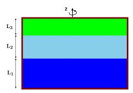
${\bf Fig.~4.67}-{\bf Three~liquids~layers~under~rotation~with~various~critical~situations.}$
