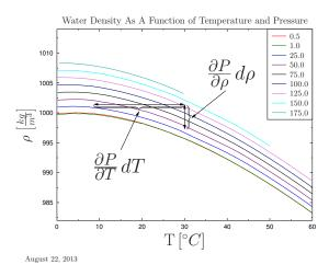
**Fig. 1.15** – Water density as a function of temperature for various pressure. This figure illustrates the typical situations like the one that appear in Example 1.9
