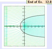
Fig. 12.14 – Source in the Uniform Flow.
