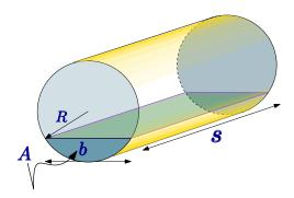
Fig. 3.8 – Segment of circular for centroid calculations.
