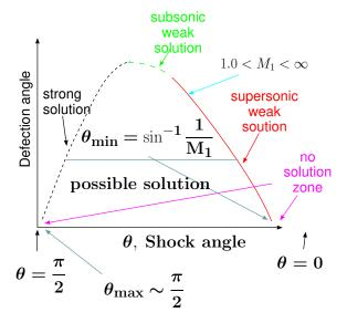
$\mbox{\bf Fig. 15.8} - \mbox{The possible range of solutions for different parameters for given upstream Mach numbers. } \\$
