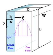
Fig. 16.16 – A diagram to explain the flood in a two dimension geometry.
