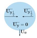
Fig. 7.3 – How to compensate and estimate the kinetic energy when averaged Velocity is zero.
