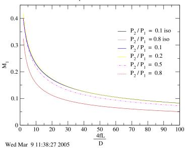
${\bf Fig.~14.38} - {\bf The~entrance~Mach~number~as~a~function~of~dimensionless~resistance~and~comparison~with~Isothermal~Flow.$
