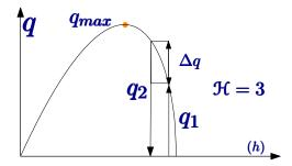
Fig. 17.21 – Flow in contraction subcritical flow. The specific energy in diagram is  $\mathcal{H}=3$  The flow at section 1 with  $q_1$  increase the flow rate per width to section 2. At section 2 now the flow rate is given and with specific energy  $\mathcal{H}$  all the parameters can be found. For example in
