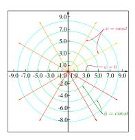
**Fig. 12.7** – Streamlines and Potential lines due to Source or sink.
