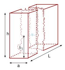
Fig. 4.57 – Cubic body dimensions for stability analysis.
