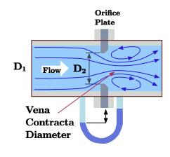
Fig. 11.15 – Orifice Plate inserted into pipe to be used measurement of flow rate.
