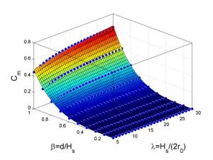
${\bf Fig.~13.9} - {\rm Added~mass~for~vertical~cylinder~moving~at~liquid.~The~parameters~shown~in}$ the figure  $\lambda$  is ratio of the diameter cylinder and of the total length, and  $\beta$  is ratio of the total length to wet length similar to density ratio.
