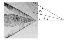
Fig. 15.11 – Oblique shock occurs around a cone. This photo is courtesy of Dr. Grigory Toker, a Research Professor at Cuernavaco University of Mexico. According to his measurement, the cone half angle is 15° and the Mach number is 2.2.
