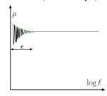
**Fig. 1.2** – Density as a function of the size of the sample.
