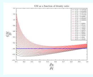
Fig. 4.58 – GM of Rectangular shape with various dimensions.
