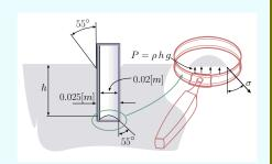
Fig. 1.19 – Glass tube inserted into mercury.
