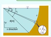
Fig. 4.28 – Calculations of forces on a circular shape dam.
