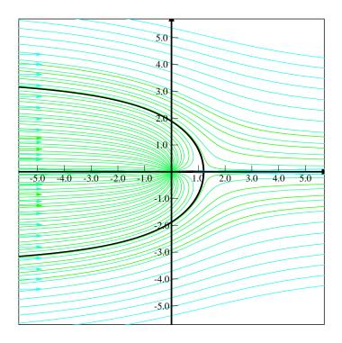
Fig. 12.20 – Uniform flow with a sink.
