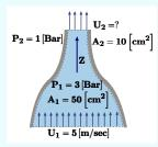
**Fig. 6.3** – Nozzle schematic for the discussion on the forces and for example 6.3.
