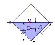
**Fig. 4.47** – Cubic on the side (45°) stability analysis.
