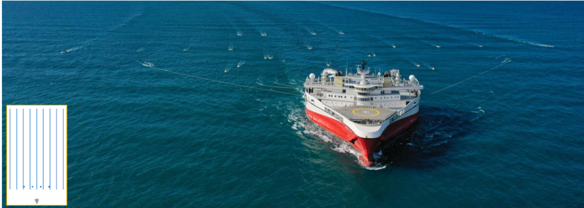
Figure 3: Ramform Tethys acquiring a high-resolution CCS baseline survey for the Northern Endurance Partnership offshore UK in 2022. The configuration consisted of 11 multisensor streamers with 50m separation and a wide quad source that was towed over the front end of the streamer spread. The resulting nominal acquisition bin size was 6.25m x 6.25m.
