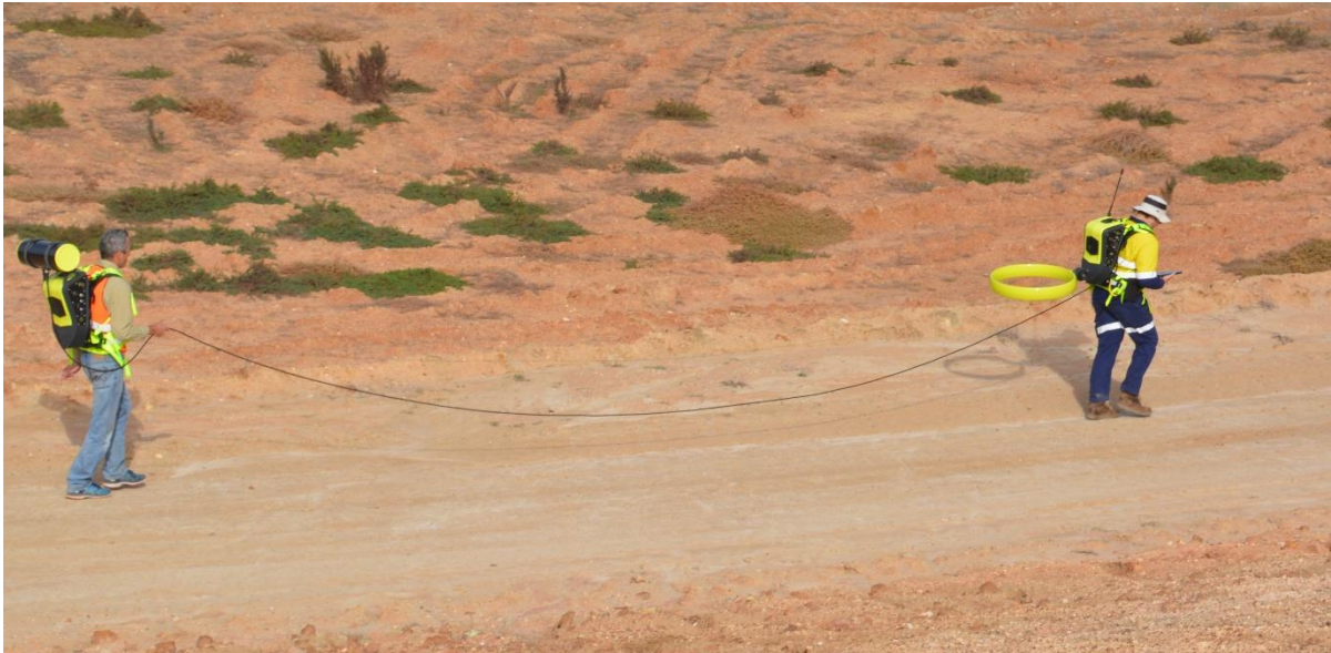
Figure 1. Loupe system deployed at mine site for TSF investigations. Data is collected at walking pace.
