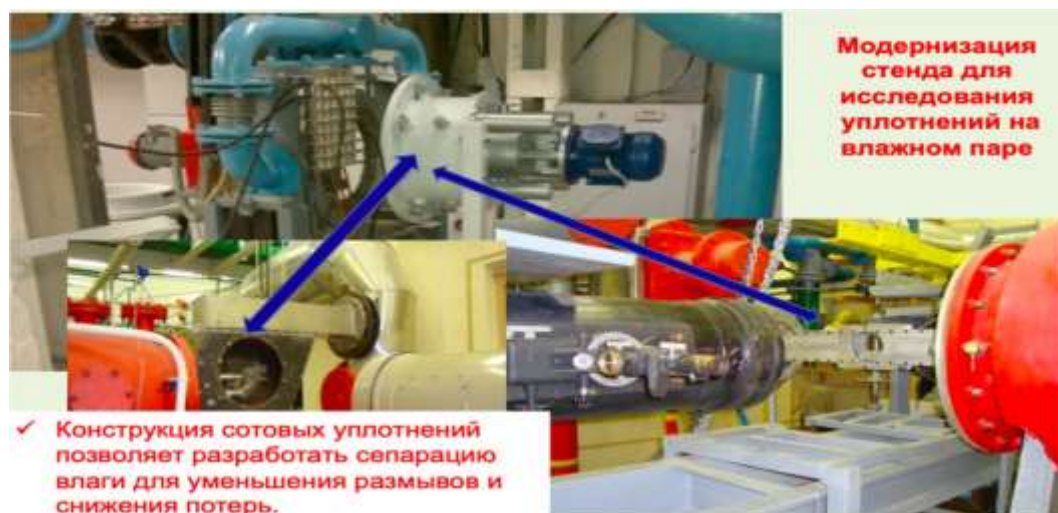
Fig 3. Stand for testing models of seals
