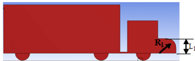
Fig. 8. A standard heavy truck model with FFRR definitions as FFRR = [R_1/L_1] .
