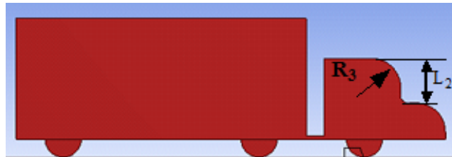
Fig. 14. A standard heavy truck model with TFRR = [R_3/L_2] , [0, 0.2, 0.3, 0.6 and 0.8] MFRR=0.2 and FFRR=0.8.
