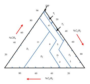
Legend: PD = partial discharge T1 = thermal fault less than 300°C T2 = thermal fault between 300°C and 700°C T3 = thermal fault greater than 700°C D1 = low energy discharge (sparking) D2 = high energy discharge (Arc) DT = mixture of thermal and electrical faults
