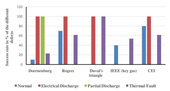
Figure 4:- Success rate of the various defects according to conventional methods.
