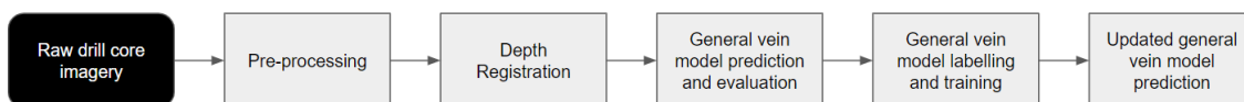
Figure 1. Overview of the steps to predict and extract vein segmentation area and percentage from drill core imagery.
