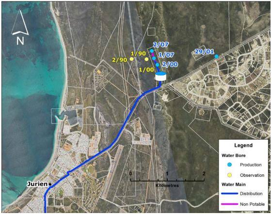
Figure 1. Satellite image with production and monitoring bores, and water infrastructure.
