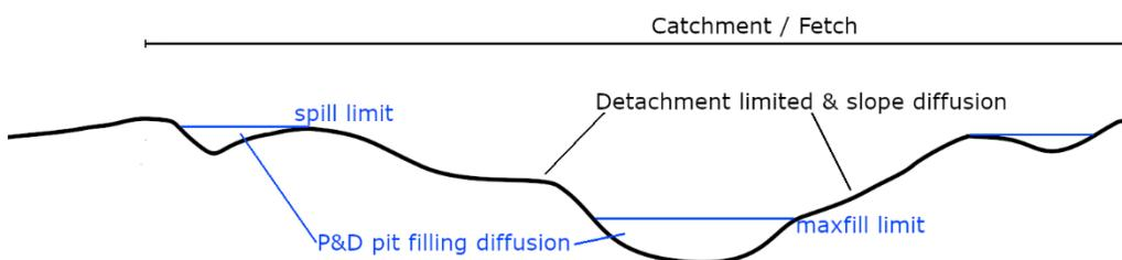
Figure 3: Schematic describing operation of detachment limited and pit-filling equations in Badlands.
