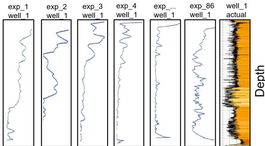
Figure 2: Comparison between lake level extracted from multiple experiments against gamma log at well location.
