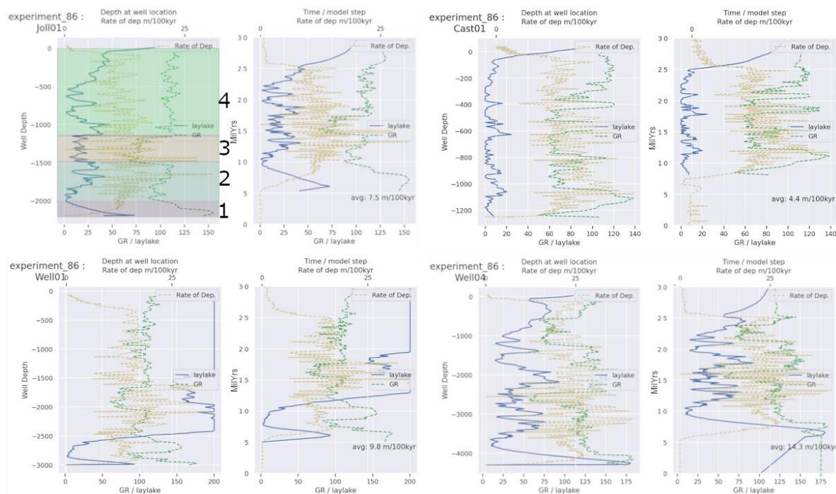
Figure 4: Lake level and gamma ray log plots at each of the 4 wells from the selected experiment. the Joll01 well shows the model phases based on the variations in lake level, sediment supply and landscape evolution.
