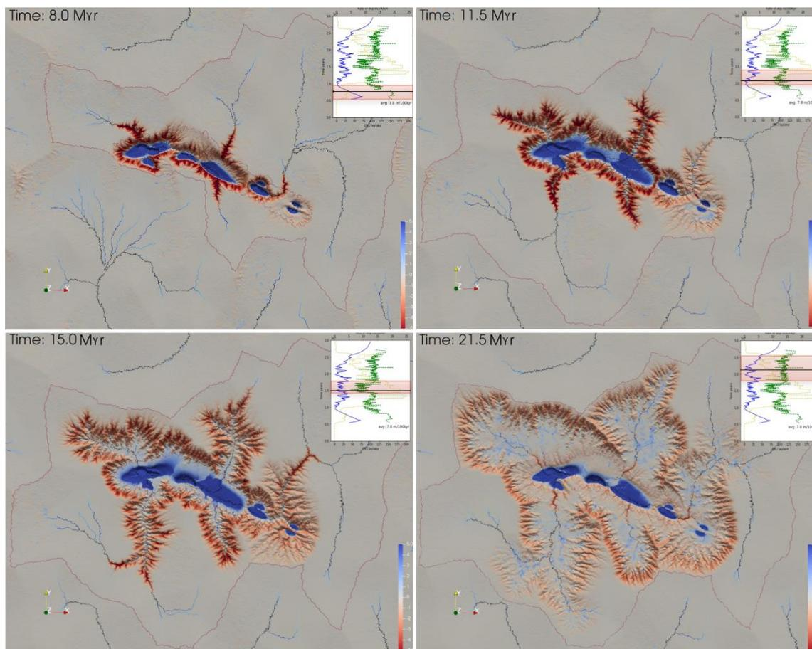
**Figure 5: Topographic surface examples during each phase. Erosion (red) and deposition (blue) over a 100,000 year time step. Insets are lake level and gamma log plotted against time of deposition with the corresponding time highlighted in red.**
