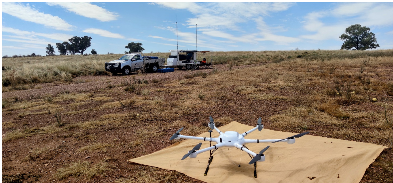
Figure 1. Hexacopter drone used in the survey with RTK GPS enabled.
