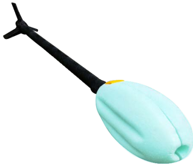
Figure 3. Image of the magnetometer bird, with the GPS mounted in the nose.
