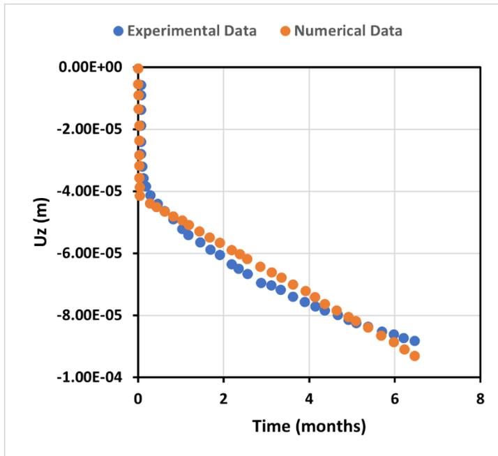
**Figure 7 Comparison of axial displacement  $u_z$  evolution with time of rock salt from numerical simulation and laboratory data under uniaxial compression.**
