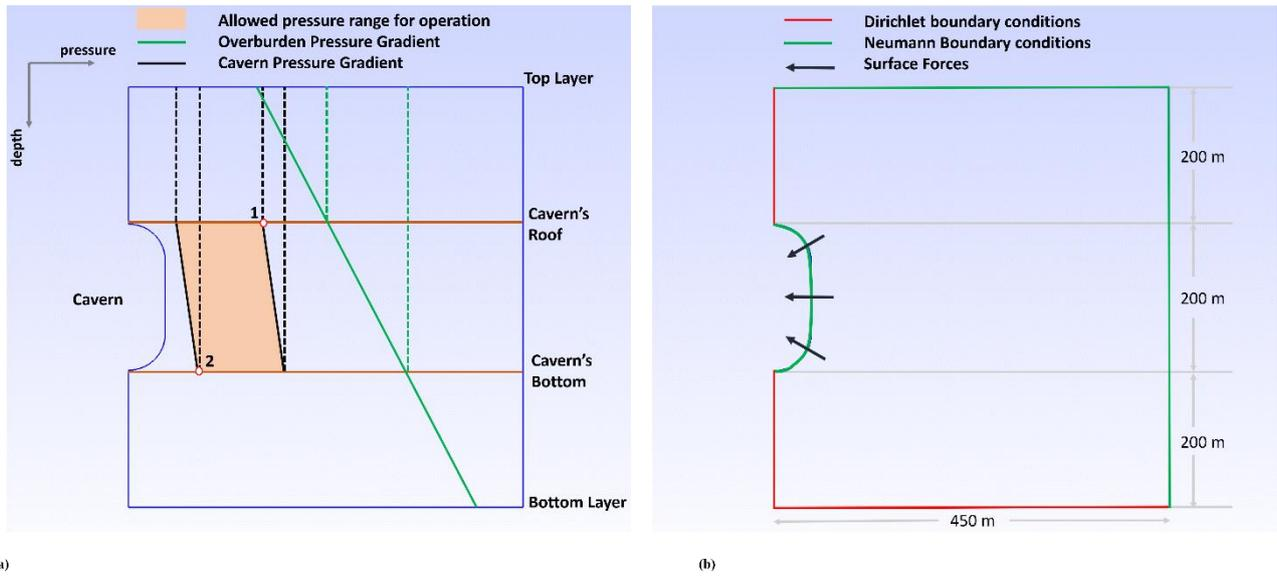
**Figure 4. The pressure gradient and safe pressure range used for numerical simulation in the salt deformation numerical study (left) and applied boundary conditions (right) for both test cases. The depth of topmost salt layer from the surface is 600 m.**
