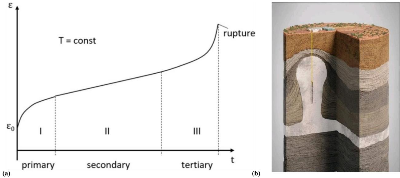
**Figure 1. (a) Creep response of a material (left) showing three stages of creep with an initial elastic deformation of  $\epsilon_0$  under (b) example of geological structure of salt dome (taken from GA, 2022 LinkedIn page).**
