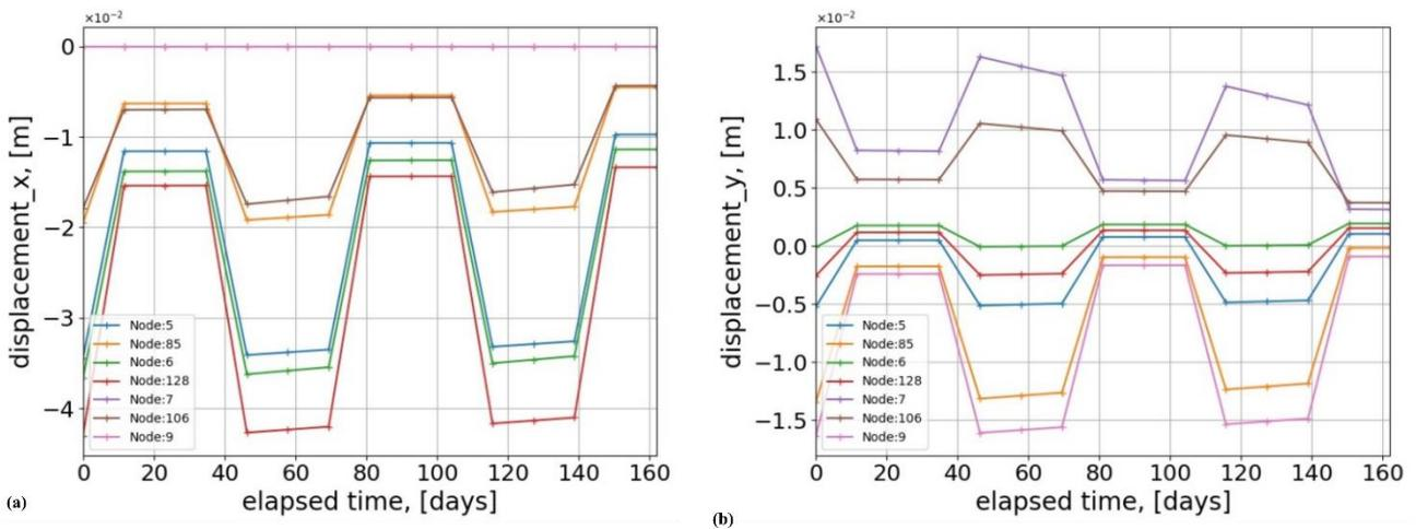
Figure 6. Creep under cyclic loading: (a) horizontal ( $u_x$ ) and (b) vertical displacement ( $u_y$ ) evolution with time.
