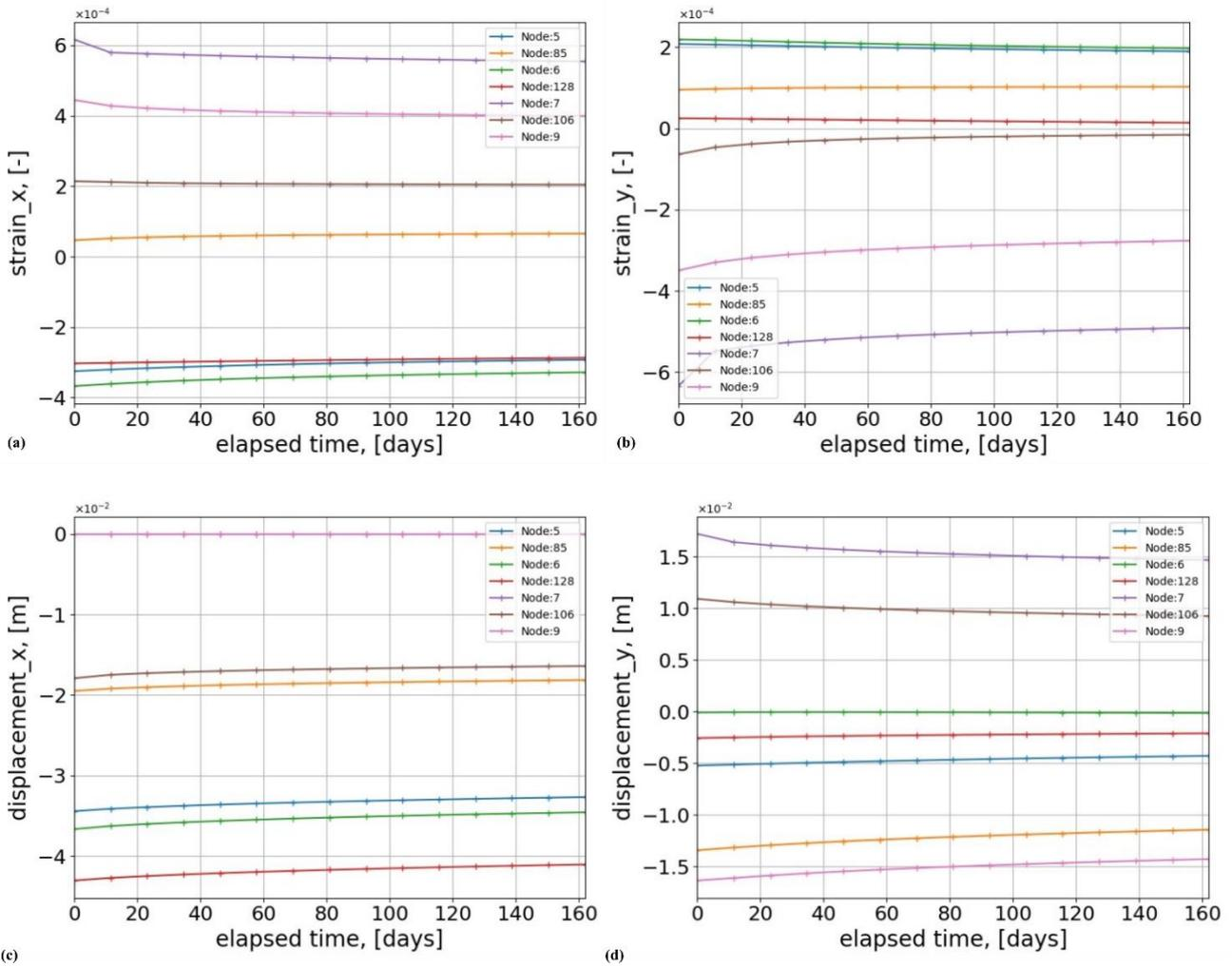
Figure 5. Creep under monotonic loading: (a, b) strain rate along radial and axial direction respectively and (c, d) horizontal and vertical displacement evolution with time respectively.
