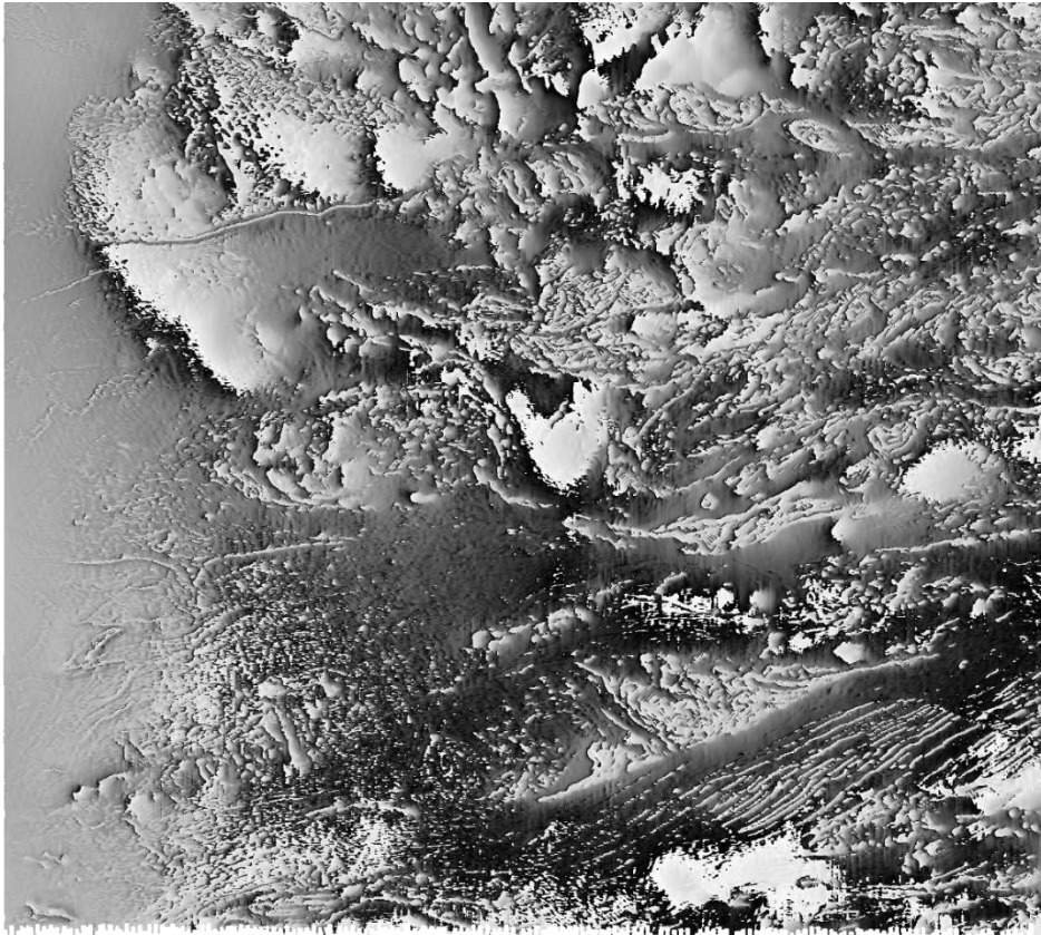
Figure 6. Cauchy Third order vertical gradient, after trend gridding, decorrugation & RTP, Units nT/m 3 .
