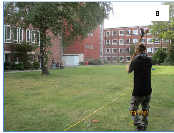
Figure 9. Data acquisition. A: placing a geophone with polar coordinate; B: Shot by a sledgehammer (linear array).
