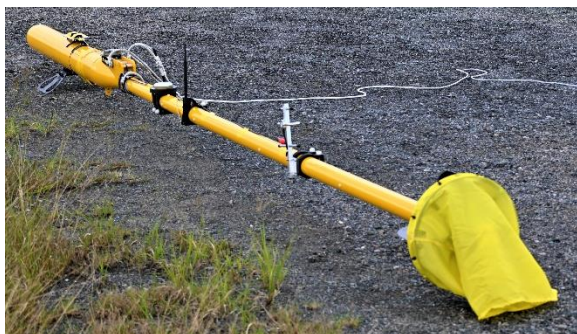
Figure 2. Gap Geophysics Australia “Generation 2” HeliSAM bird.
