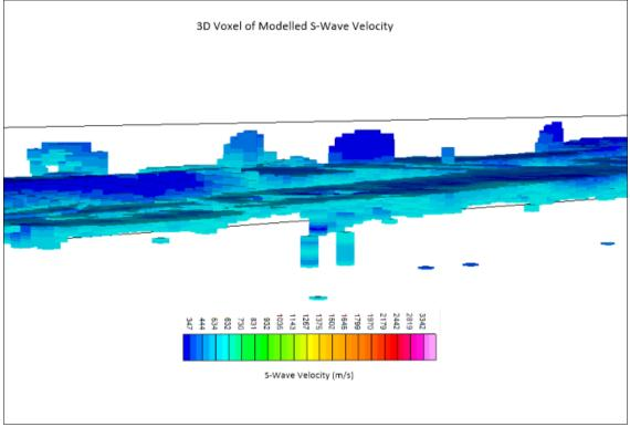
Figure 2. Modelled examples of low velocity areas extending with depth. Velocity cut off is shown at 650m/s.
