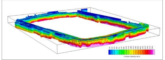
Figure 1. 3D voxel outlining all modelled seismic velocities (Vs) to 30m. Low velocities (250m/s) are shown in blue, increasing velocities are stretched to pink (2800m/s)
