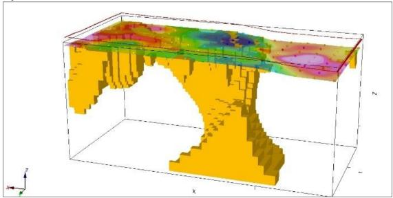
Figure 3. Modelled example of a low velocity area extending along the Y scale, draping a gravity anomaly on the X scale. Correlation of both datasets outlines an area of interest extending with depth.
