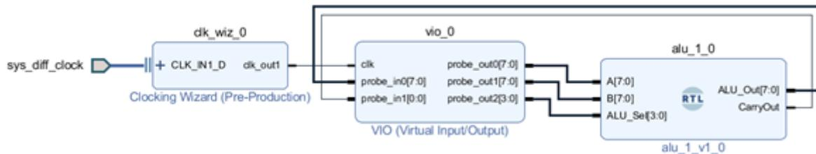
Figure 10: Generating Block design of FPGA based ALU
