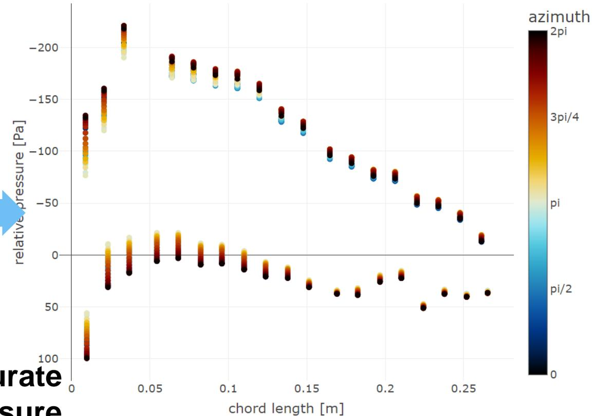
... to accurate pressure distribution on a wind turbine blade?
