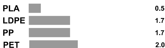
Figure 5. CO 2 equivalent emissions in kg per kg of polymer—cradle to gate. Adapted from BioApply.
