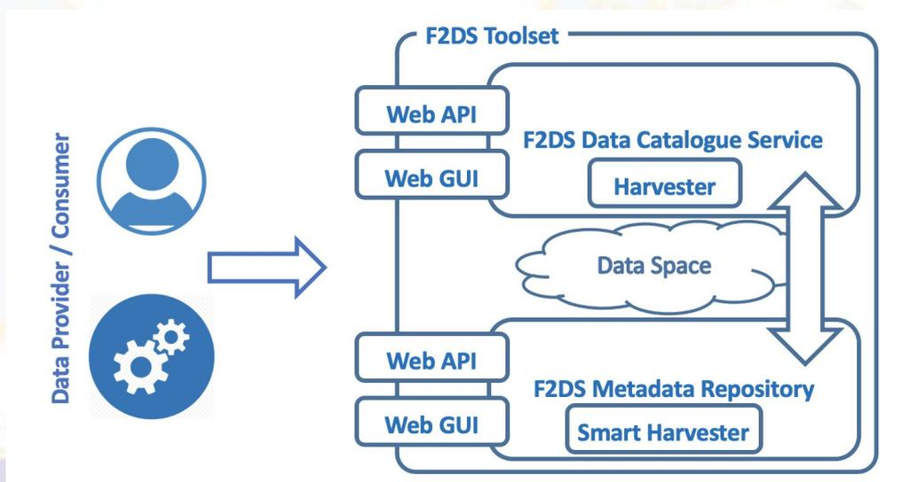
Figure 1 F2DS workbench Overall Architecture
