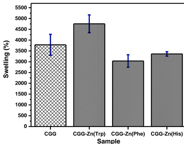
**Figure 2.** Maximum swelling capacity (%) of the composite hydrogels
