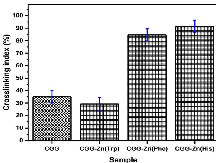
**Figure 3.** Crosslinking index (%) of the composite hydrogels
