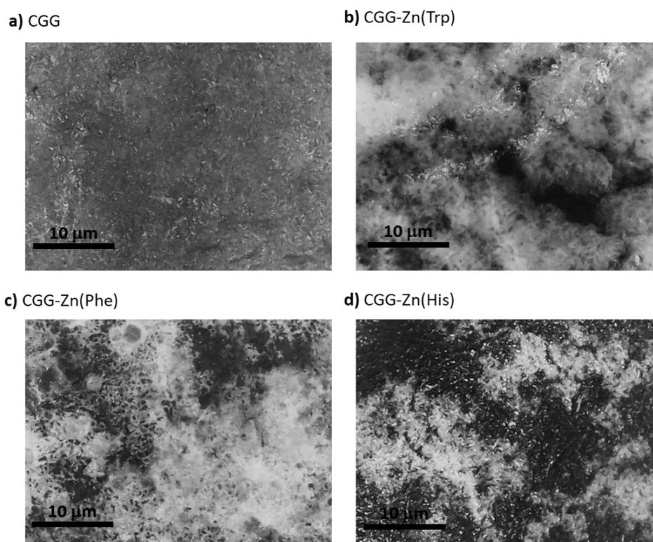
**Figure 5.** SEM micrographs of CGG hydrogel and CGG-Zn(AA) composite hydrogels
