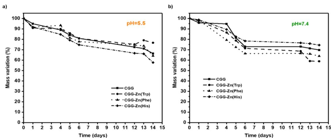
**Figure 4.** Degradation profiles in hydrolytic media (pH=5.5 and pH=7.4) of the composite hydrogels
