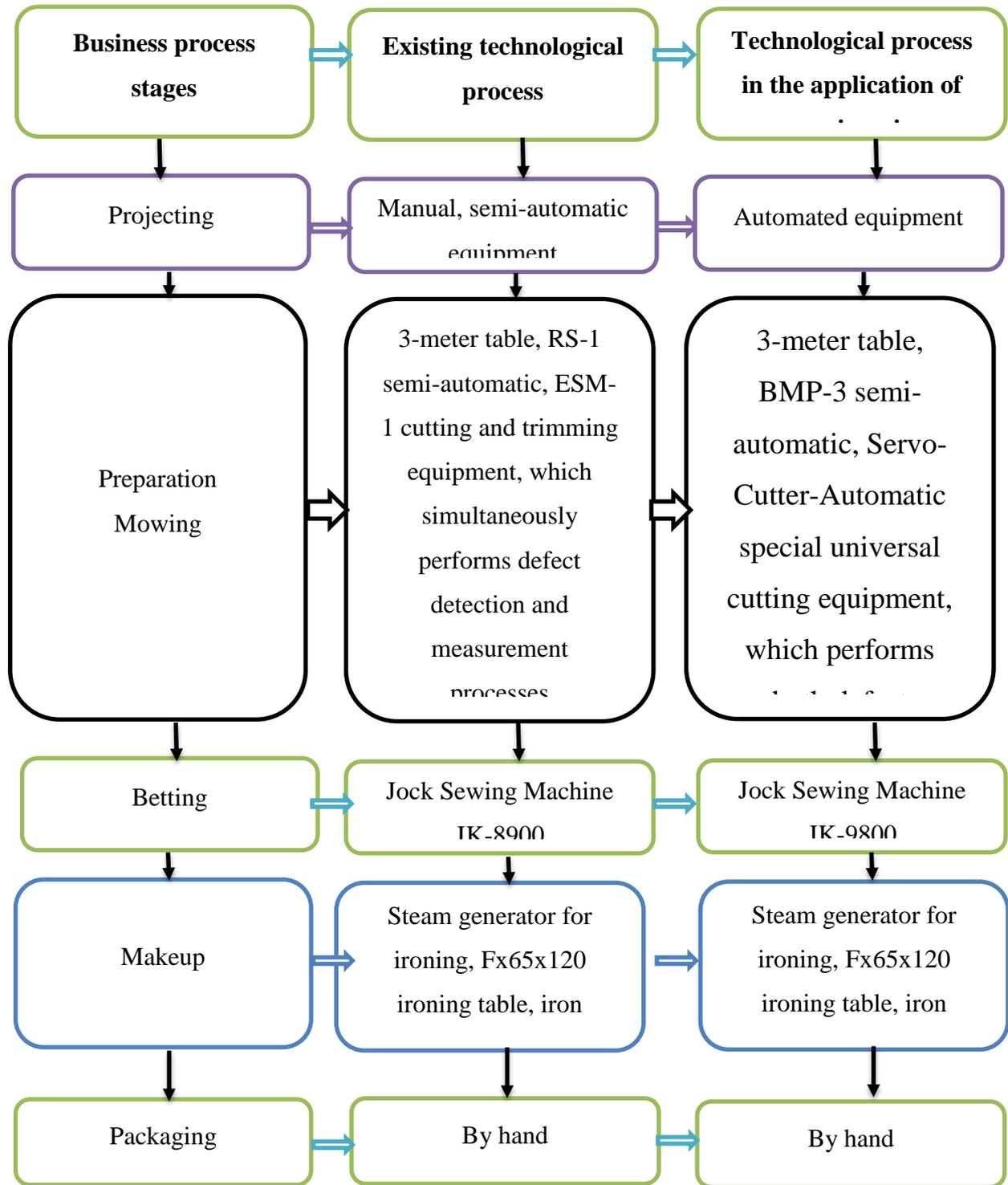
**Figure 2. Scheme of technological chain stages of reengineering the main business process in a sewing enterprise<sup>2</sup>**
