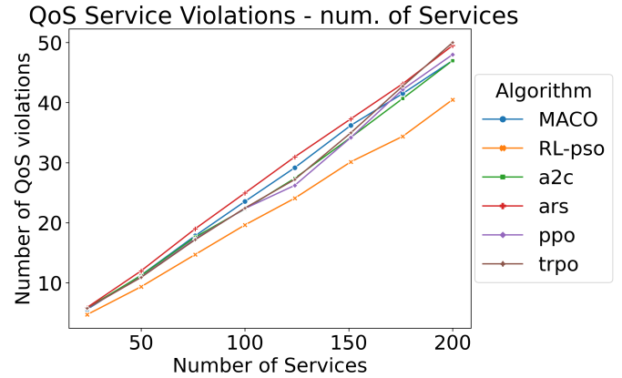
Fig. 4. Aggregated mean for the number of Quality of Service violations for N=500 experiments.
