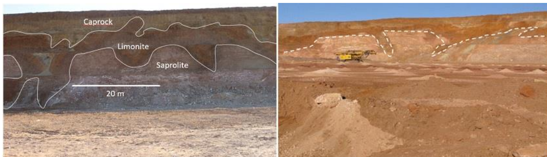
Figure 1. Photograph of pit wall showing complexity of main material interfaces (left). Note 20 m scale bar that represents current grade control drill spacing. Pre-existing structures control localised, deep weathering, illustrated by the abrupt limonite features traced by the dashed white line (right).
